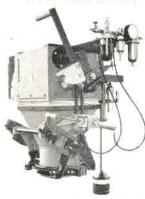
Automatic, Air Operated — footpedal control leaves both hands free to apply bags . . . gives increased bagging speed over manual types; toggle action locks clamps in either open or closed positions; rubber inserts (adjustable) in clamps seal bag around spout to keep dust in and prevent slippage. (Cam-grip bagholder is standard).
