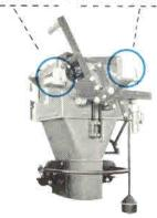
Five-figure setback counter registers number of bags filled. Direct-connected to gate operating handle . . . registers one count each time bag is filled . . . can be returned to zero at the end of each run. Conveniently mounted at operator height.
